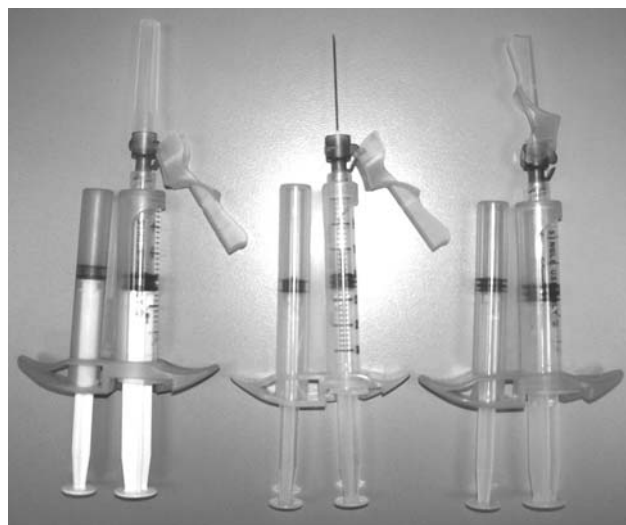
Fig. 1 Safety needle on the reciprocating procedure device (RPD). A BD safety needle with an off-axis rotating safety sheath was chosen as the safety device to reduce needlestick injuries and is shown here mounted on the RPD safety device. The BD needle comes with two sheaths ( left RPD ), a conventional sheath that is removed to expose and then use the needle ( middle RPD ), and then a lateral rotating sheath that is pushed with the finger and encloses and inactivates the used needle ( right RPD )
